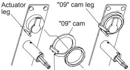
Cylinder nut Notch of cam Due to individual cam configurations and cylinder lengths, the leg of the "09" cam may have to be bent slightly to function properly. 95054195 "09" Pack
