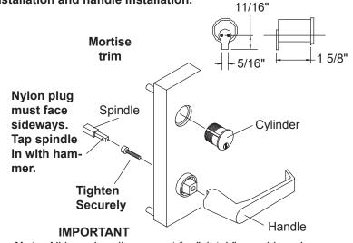
Note: All lever handles except for "clutch" are shipped unattached. To install; Place handle in desired position and attach with allen screw located in back of trim plate. 5/32" Allen wrench required. To change hand on "clutch" trim rotate and "break" lever around to desired hand.
